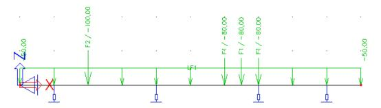
The user can set the limits to move the supports, each variant is calculated and reactions are evaluated. The goal function can be a simple formula, which calculates the sum-of-squares of deviations from an average value of reaction.
