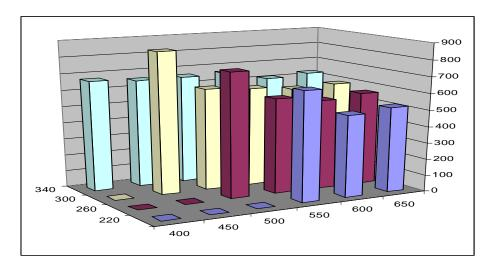
The optimal shape of the cross-section was found 600x220 mm.
