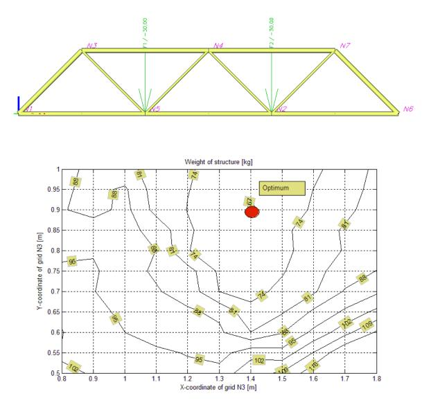
The optimal shape of the structure is like this :
