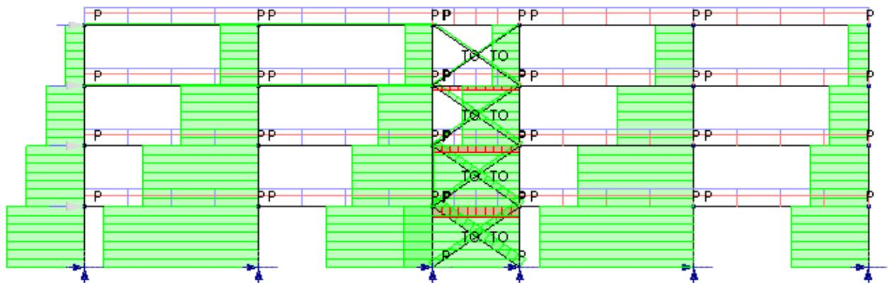
The diagonals, columns and beams of the braced bay form a closed system in which vertical loads are shared between the columns and diagonals according to their stiffness. The second stage of the simple analysis removes all the diagonals leaving the frame as a sway mechanism – and a (spurious) failure is reported.
