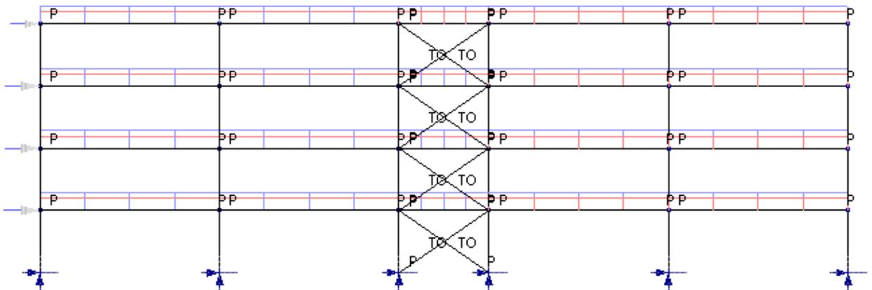
Under horizontal loads acting alone, the bracing pairs are alternately in compression and tension and application of the simple directional analysis procedure causes the 'windward diagonals' to be removed and the 'leeward diagonals' to transmit all the wind loads to the foundation supports – no problem. However in a typical load combination the gravity loadings may be dominant causing all the diagonals to be in compression under normal linear analysis as shown below:
