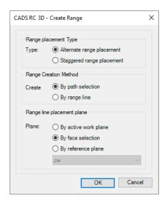
Range Placement Type - Use the Rebar Range Placement *Create Range* command to create a Staggered group of rebar from a single bar or Alternate group of rebar from two single bars in the model.
