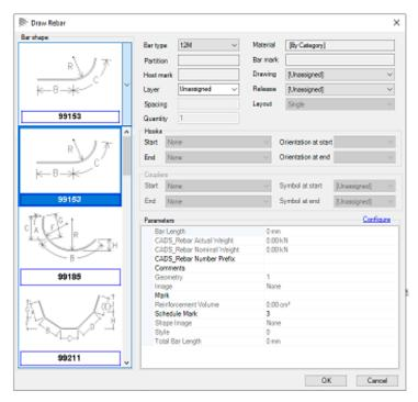
The CADS Rebar Shapes that are deployed along with the installation are either not possible or difficult to create using Revit's native rebar shape family file.
